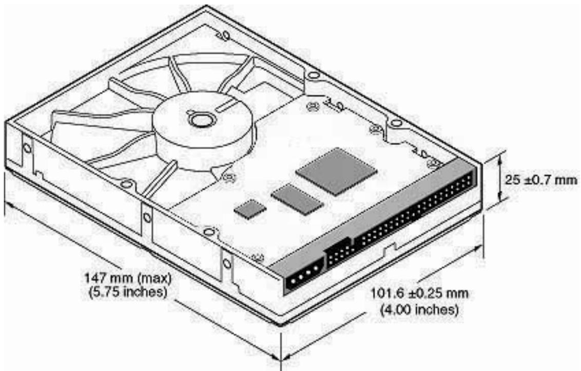
**Figure 3-1** Mechanical Dimensions of Maxtor DiamondMax 10 Hard Disk Drive
