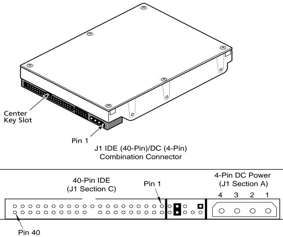
**Figure 3-6** J1 DC Power and ATA Bus Combination Connector
