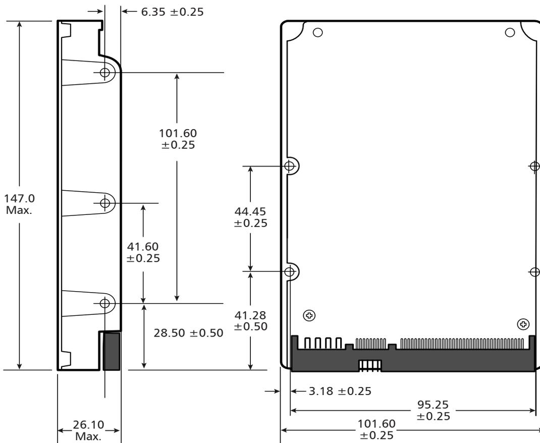
**Figure 3-7** Mounting Dimensions for the Maxtor DiamondMax 10 Hard Disk Drives
